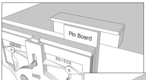
Use Support as shown to set height of pin board in vise (1-1/4" above bench top).
